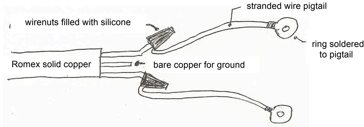
Note: Solder – there are two types of solder typically available, one for electrical use and one for plumbing. Use electrical, rosin-core solder.
